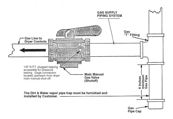
The dryer and its individual shutoff valve must be disconnected from the gas supply piping system during any pressure testing of that system at test pressures in excess of 1/2 psi (.04 bar).
