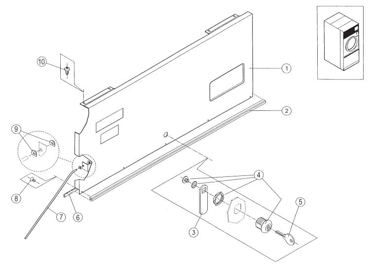
CSA-01582WH Complete control door assy. - Simple microprocessor CSA-01407WH Complete control door assy. - Double Timer
